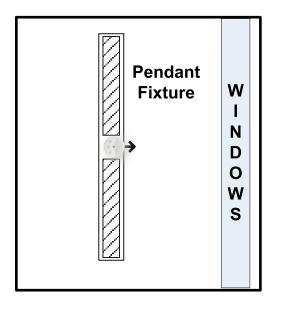
**Option 2:** If the fixture is **perpendicular** but one side is far enough from the window (see page 11) you can place the sensor as shown below.
