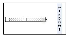
**Option 3:** You can also place the sensor in the same vertical plane as the pendant. This approach may work for pendant fixtures perpendicular to the window, depending on the fixture design.
