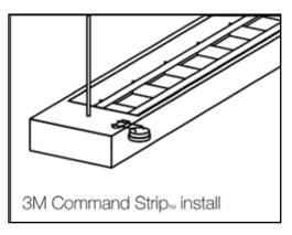
How to place the sensor on a pendant fixture using Option 3.
